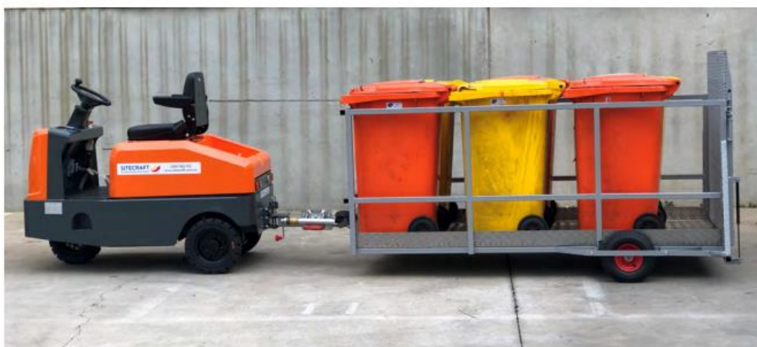
ST3000-AC tow tug complete with 6 x 250AH heavy duty batteries
